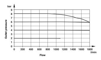
Flow from 1 to 2, Inlet pressure 7 bar
